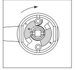
2. Holding lever securely, rotate rose assembly clockwise lockwasher.
