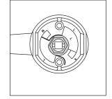
7. Reinstall lockwasher and nut. Tighten nut and then back off slightly until rose assembly rotates freely under plate. Bend up one tab of lockwasher against nut.
