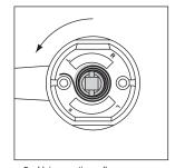
3. Using caution, allow rose assembly to rotate counterclockwise to relieve spring tension.
