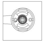
4. Remove spring and reinstall with spring hook on opposite side of post.
