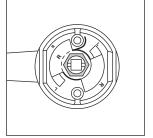
Holding lever as shown, bend tab of lockwasher back flat Remove nut
