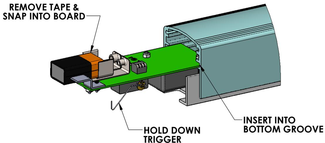
3. Mount the "dogged" Exit Device, with the Alarm Board encased in the push bar, to the door frame. Tighten the 2X 1/4-20 Mounting Screws.
