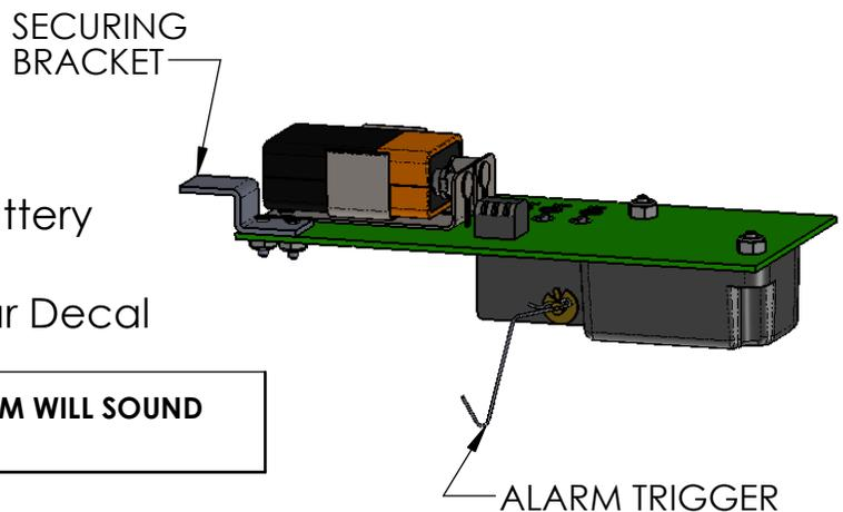
(NOTE: If shipping the exit device loose (Not installed on a door), be sure to secure the Alarm Board so that it will not fall out during handling.)
