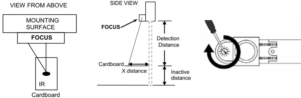
NOTE: The Focus 2 is not configured to allow angle adjustment. The Focus 2 only allows for height adjustment.
