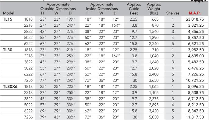
\*Outside depth dimension doesn't include dial, handle and hinge. • When shipping add 100-150 lbs. for safe skid to weight.
