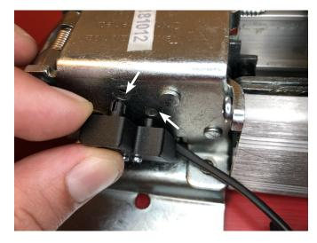
**8.** INSTALL (1) 40266 SCREW INTO TOP HOLE ON LBM BRACKET TO SECURE BRACKET TO EXIT DEVICE HEAD.
