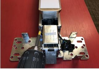
**6.** PUSH THE TWO TABS ON THE LBM BRAKET INTO THE EXISTING HOLES IN THE EXIT DEVICE HEAD.
