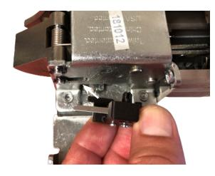
7. CONFIRM SWITCH ARM IS UNDERNEATH RIM LATCH PIN. INSTALL (1) 40266 SCREW INTO TOP HOLE ON LBM BRACKET TO SECURE BRACKET TO EXIT DEVICE HEAD.
