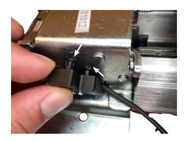
8 INSTALL (1) 60754 CAP ON TO LATCHBOLT ROLL PIN.
