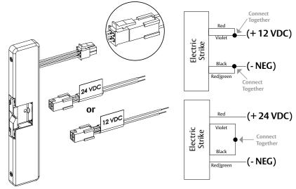
Diagram 3: Fail Secure Operation
