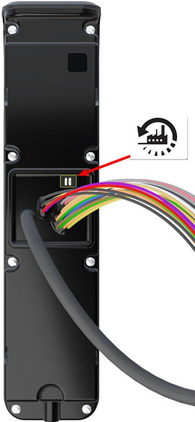
4. With power supplied to the reader, short the contacts together using a suitable metal object.
