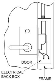
Electric Actuator. Solenoid points up when actuator is used with:
