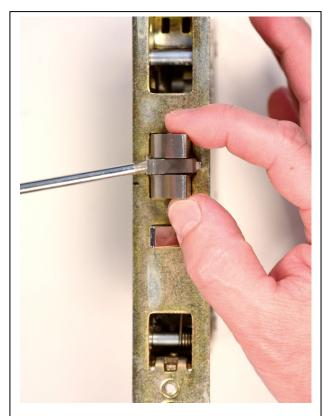
• Tilt the latch cam and pull the latch straight out from the lock case.
