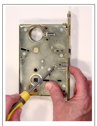
Flip the lock body over and remove the second latch screw.
