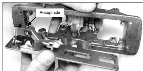
4. Turn back plate 180° so that the receptacle is in the bottom position.
