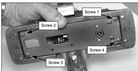
1. The underside of the model 1100 is shown, with four (4) screws that must be removed.
