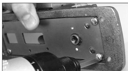
2. Remove all 4 screws with a slotted screwdriver. Place screws aside.
