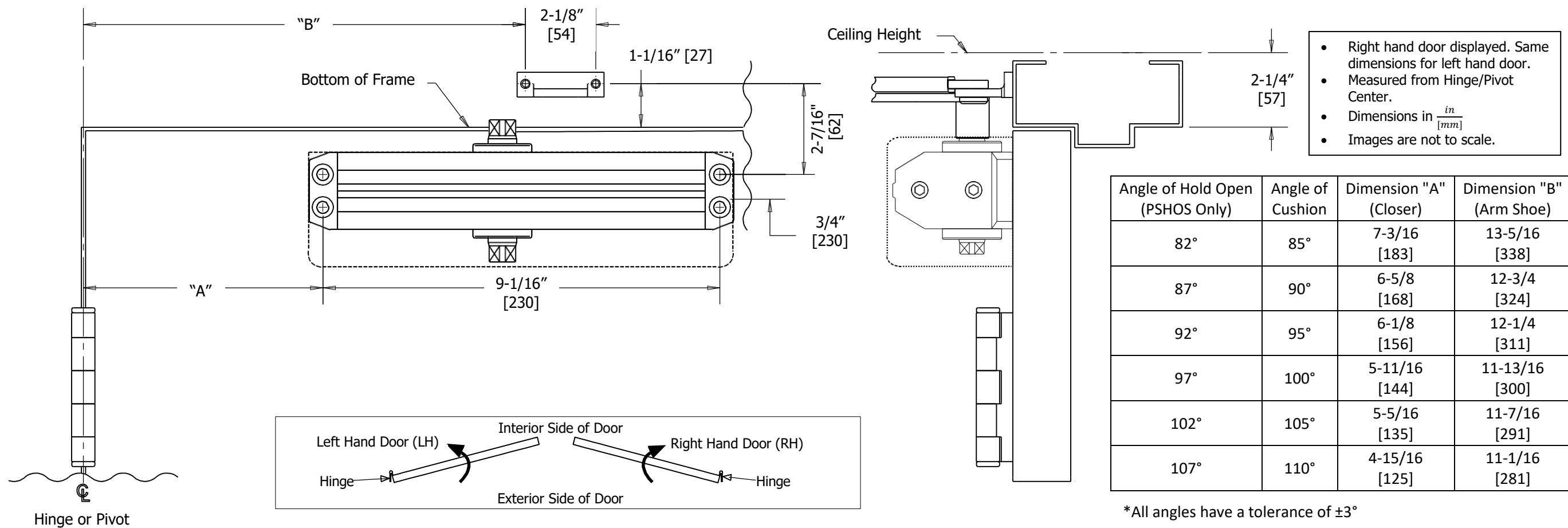
\*All angles have a tolerance of  $\pm 3^\circ$
