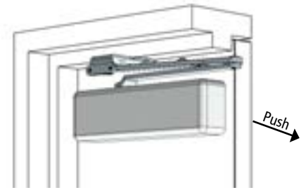
Parallel Arm (Push Side) Permits 180° maximum opening
