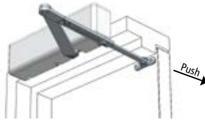
Top Jamb (Push Side) Permits 120° maximum opening
