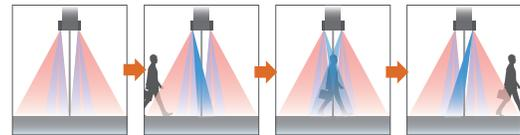
Whole presence detection capability OA-FLEX T can use detection area as presence detection area and possible to utilize for various applications.
