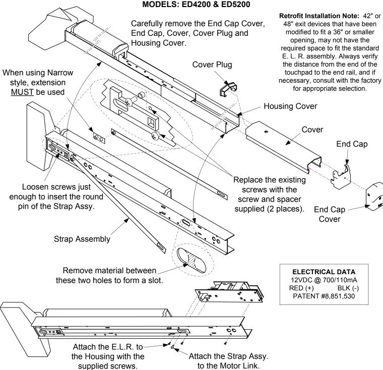
Replace Housing Cover, Cover with Plug, End Cap and the End Cap Cover.
