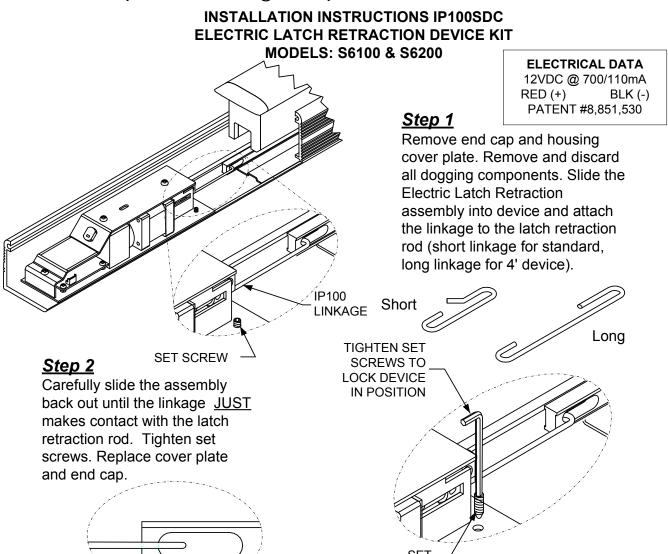
**Retrofit Installation Note:** 42" or 48" exit devices that have been modified to fit a 36" or smaller opening, may not have the required space to fit the standard E. L. R. assembly. Always verify the distance from the end of the touchpad to the end rail, and if necessary, consult with the factory for appropriate selection.
