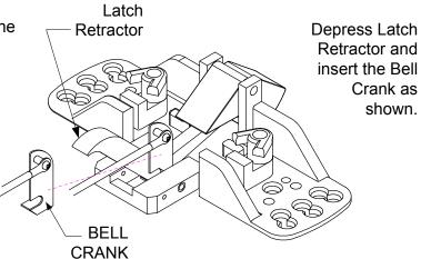
Mount the ELR assembly in the device by positioning the assembly close to the edge of the rail (leave enough room for the End Cap). Drill and tap an 8-32 hole centered on the rail, and attach ELR to rail with supplied screw. Run the cable through the ELR Clevis Block and Cable Sleeve. Install the device to the door.
