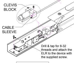
ELECTRICAL DATA 12VDC @ 700/110mA RED (+) BLK (-) PATENT #8,851,530 **Energize** the ELR assembly, then pull the cable so that it retracts the latch far enough to clear the strike. Hold the cable in position and secure the set screw firmly on the clevis block, so that the Cable Sleeve secures the cable in block. Test operation and re-attach access cover (NOTE: Access Cover can **NOT** go back on the same way as it came off. It must be rotated 180 degrees).
