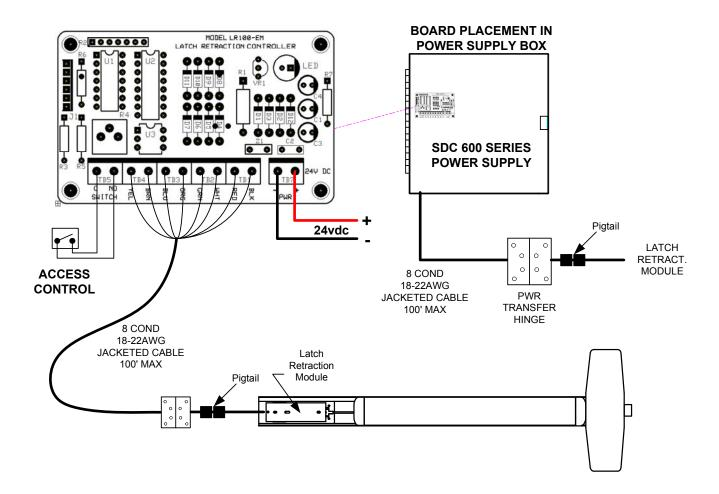
Retrofit Installation Note: 42" or 48" exit devices that have been modified to fit a 36" or smaller opening, may not have the required space to fit the standard E. L. R. assembly. Always verify the distance from the end of the touchpad to the end rail, and if necessary, consult with the factory for appropriate selection.
