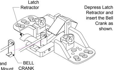
Run the cable through the ELR Clevis Block and Cable Sleeve. Install the device to the door. Mount the ELR assembly in the device by positioning the assembly close to the edge of the rail. Use the mounting tab from the exit device to secure the ELR to the base. Once the assembly is secure then use a 7/64 drill bit to drill out the inserts and use the supplied screws to fasten kit to the device and door.
