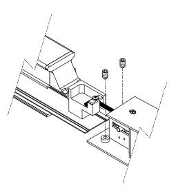
**Retrofit Installation Note:** 42" or 48" exit devices that have been modified to fit a 36" or smaller opening, may not have the required space to fit the standard E. L. R. assembly. Always verify the distance from the end of the touchpad to the end rail, and if necessary, consult with the factory for appropriate selection.
