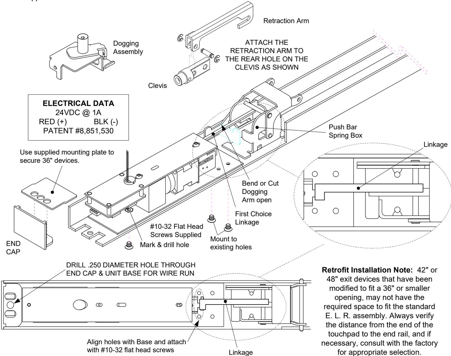
When retrofitting to existing vertical rod devices, adjustment of the rods is required for proper operation of the Electric Latch Retractor. Once the unit is properly installed, energize it so the push pad is dogged down, then reconnect the vertical rods to the device and make the proper adjustments.
