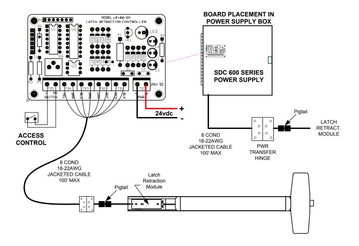
**<u>Retrofit Installation Note:</u>** 42" or 48" exit devices that have been modified to fit a 36" or smaller opening, may not have the required space to fit the standard E. L. R. assembly. Always verify the distance from the end of the touchpad to the end rail, and if necessary, consult with the factory for appropriate selection.
