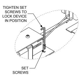
**Retrofit Installation Note:** 42" or 48" exit devices that have been modified to fit a 36" or smaller opening, may not have the required space to fit the standard E. L. R. assembly. Always verify the distance from the end of the touchpad to the end rail, and if necessary, consult with the factory for appropriate selection.
