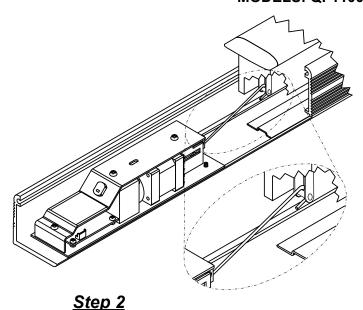
Carefully slide the assembly back out until the linkage <u>JUST</u> makes contact with the latch retraction rod. Tighten set screws.
