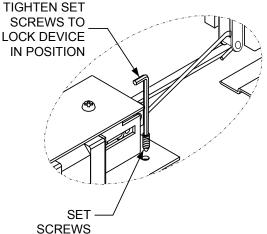
**Retrofit Installation Note:** 42" or 48" exit devices that have been modified to fit a 36" or smaller opening, may not have the required space to fit the standard E. L. R. assembly. Always verify the distance from the end of the touchpad to the end rail, and if necessary, consult with the factory for appropriate selection.
