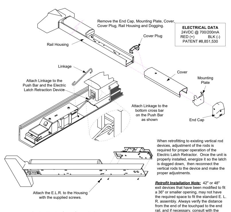
Replace Housing Cover, Cover with Plug, End Cap and the End Cap Cover.
