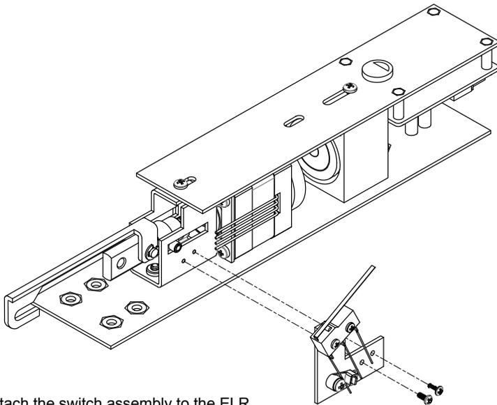
Attach the switch assembly to the ELR unit with the supplied screws as shown.
