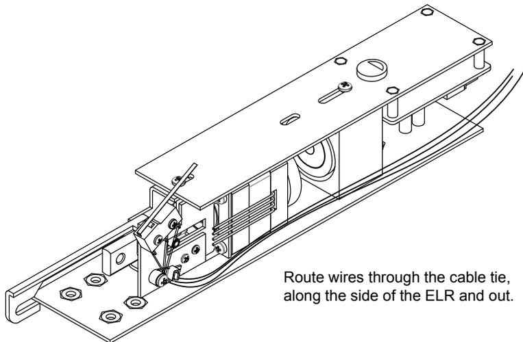
Route wires through the cable tie, along the side of the ELR and out.
