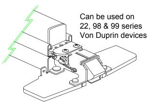
The switch wires can be routed through the bar (shown) or through the door.
