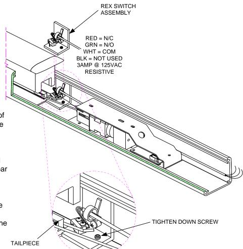
Insert switch assembly into the extrusion with the back of the angle bracket against the inside wall of the extrusion.
