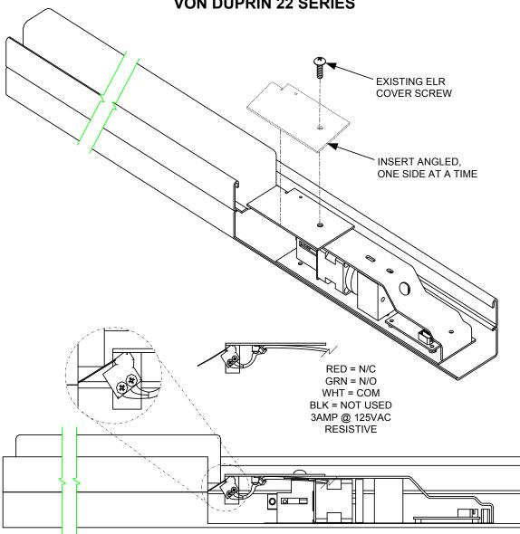
Remove and retain the existing screw on the ELR cover. Route the REX switch kit wires along the inside of the extrusion taking care not to interfere with any of the ELR components.
