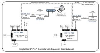
The addition of a second Ethernet port allows the IT department to save a port when connecting an additional door at the server. Installers have the potential to eliminate a long cable run to connect an additional IP device.
