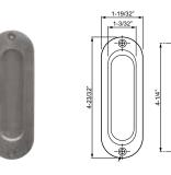
Size:  $1 \frac{9}{32}$ " W x 4  $\frac{23}{32}$ " H Depth:  $\frac{15}{32}$ " Substrate: Brass Fasteners: Exposed #6 x  $\frac{5}{8}$ " FH PH ANSI: Designed to A156.9 and A156.14 specifications and standards
