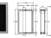
Size: 2.438" W x 3.938" H Depth: .601" Substrate: Brass Fasteners: Concealed #8 x <sup>3</sup>/4" OH PH ANSI: Designed to A156.9 and A156.14 specifications and standards
