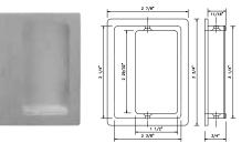
Size: 2 <sup>7</sup>/<sub>8</sub>" W x 3 <sup>3</sup>/<sub>4</sub>" H Depth: <sup>11</sup>/<sub>16</sub>" Substrate: Brass Fasteners: Concealed #6 x <sup>3</sup>/<sub>4</sub>" OH PH ANSI: Designed to A156.9 and A156.14 specifications and standards 955 Rectangle flush pull
