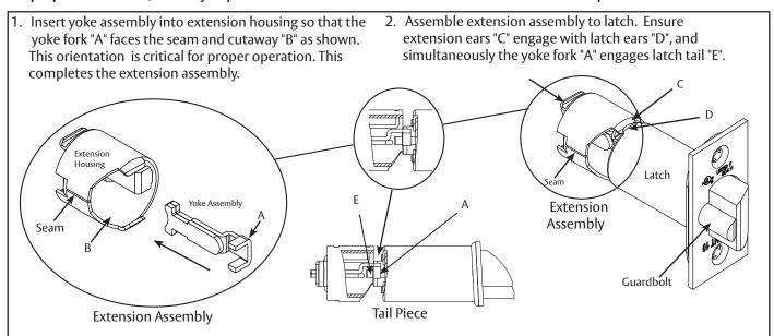
3. After assembly, the seam and cutaway "B" need to be in the same side as deadlocking guardbolt. Then assemble sleeve to hold both latch and latch extension.
