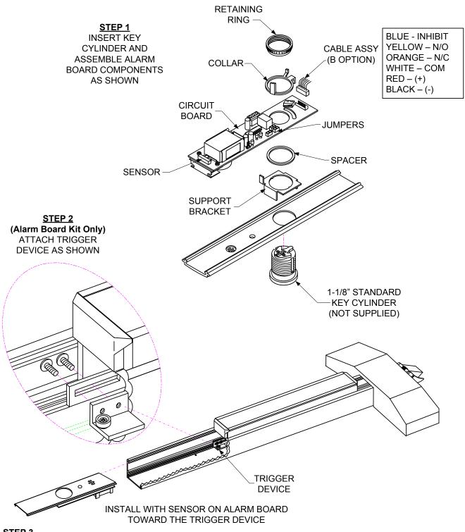
STEP 3 SLIDE ALARM BOARD ASSEMBLY INTO EXIT DEVICE
