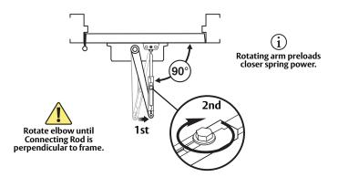
The 1130 Non Hold Open Closer - Regular Arm has now been installed. • Go to page 2 for closer adjustments and decorative cap or cover installation.
