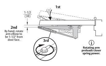
The **1130 Non Hold Open Closer - Parallel Arm Mount** has now been installed. • Go to page 2 for closer adjustments and decorative cap or cover installation.
