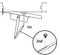
5. Preload spring and tighten forearm screw.
