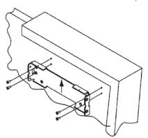
USE MOUNTING BRACKET AS DRILL THRU TEMPLATE.
