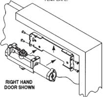
ATTACH TRACK TO STOP AT LOCATION DETERMINED FROM TEMPLATE. CUT OUT TOWARD NON-HINGE EDGE OF DOOR, USING FOUR TAMPER PROOF SECURITY SCREWS.
