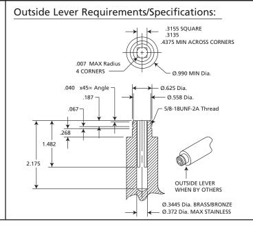
**IMPORTANT NOTE:** UNLESS OTHERWISE SPECIFIED ALL TOLERANCE TO BE + OR - .005 LEVER WEIGHT AND CONFIGURATION (center of gravity - cg) MUST NOT APPLY A MAXIMUM LEVER TORQUE THAT EXCEEDS 1.4 in-lbs.
