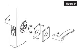
Note: To level plate, place a right angle square on the flat portion of the mounting plate.
