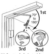
LH: Counter clockwise to tighten.
