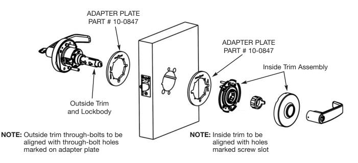
Install (1) adapter plate between door and rose assemblies (both sides) For lock installation, refer to instruction sheet A7133G
