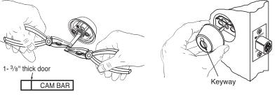
C) Install cylinder housing assembly-First assemble outside cylinder housing into outside cylinder housing collar, then insert cam bar into cam slot and position cylinder housing assembly onto door so
