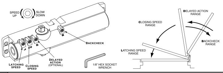
ADJUST POWER TO ALLOW DOOR TO CLOSE AND LATCH.
