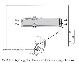
3В MOUNT FOOT BRACKET TO DOOR STOP. **CPSH SHOWN CPS SIMILAR** USF SPACER WHEN REQUIRED **IMPORTANT: USE A** MINIMUM OF 7 SCREWS.
