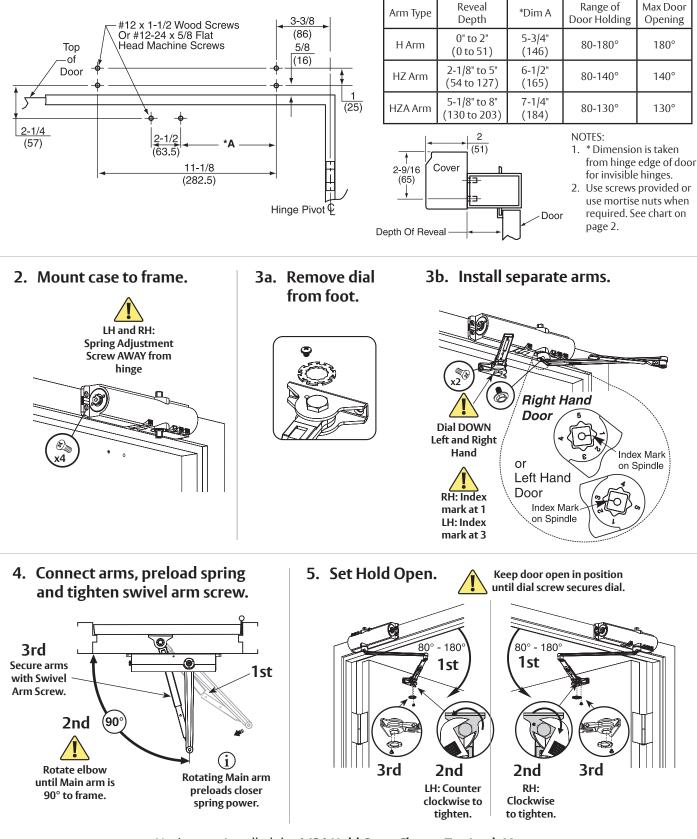
You've now installed the **1431 Hold Open Closer - Top Jamb Mount.** Go to page 7 for closer adjustments and cover installation.
