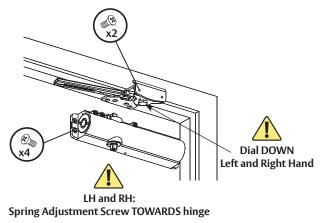
6. Rotate bottom case spindle.
