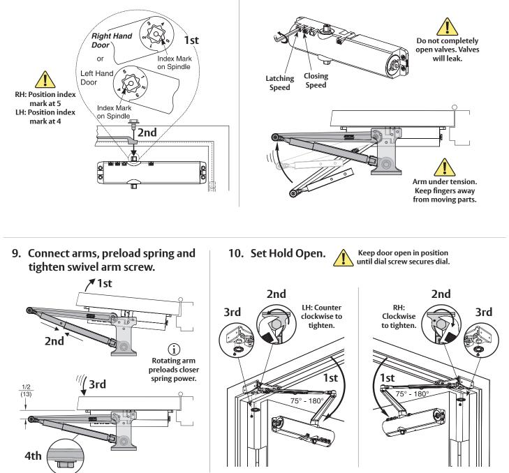
You've now installed the **1431 Hold Open Closer - Parallel Arm Mount.** • Go to page 7 for closer adjustments and cover installation.
