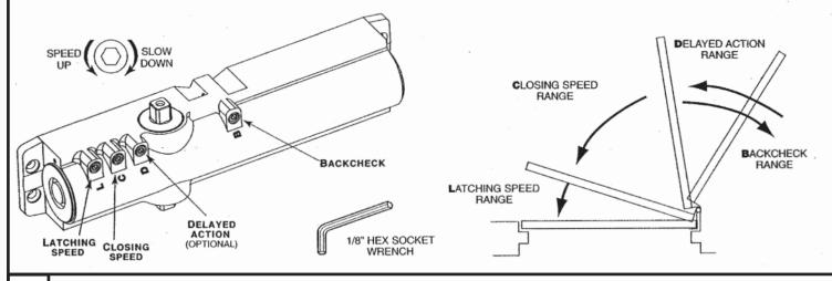
7 ADJUST POWER TO ALLOW DOOR TO CLOSE AND LATCH.
