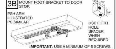
ALTERNATE: PREASSEMBLE ARM PRIOR TO ATTACHING TO STOP.
