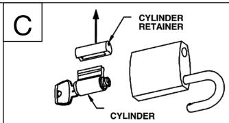
Remove cylinder retainer from cylinder for repining. Reverse steps to reassemble.
