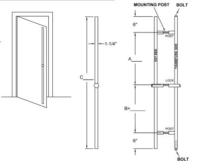
NOTE: CYLINDER MUST BE LOCATED 34"-48" ABOVE FINISHED FLOOR TO MEET ADA REQUIREMENTS. CALIFORNIA ADA REQUIRES CYLINDER TO BE LOCATED 36"-46" ABOVE FINISHED FLOOR.
