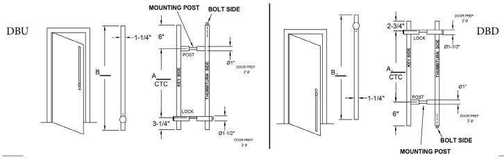
NOTE: CYLINDER MUST BE LOCATED 34"-48" ABOVE FINISHED FLOOR TO MEET ADA REQUIREMENTS. CALIFORNIA ADA REQUIRES CYLINDER TO BE LOCATED 36"-46" ABOVE FINISHED FLOOR.
