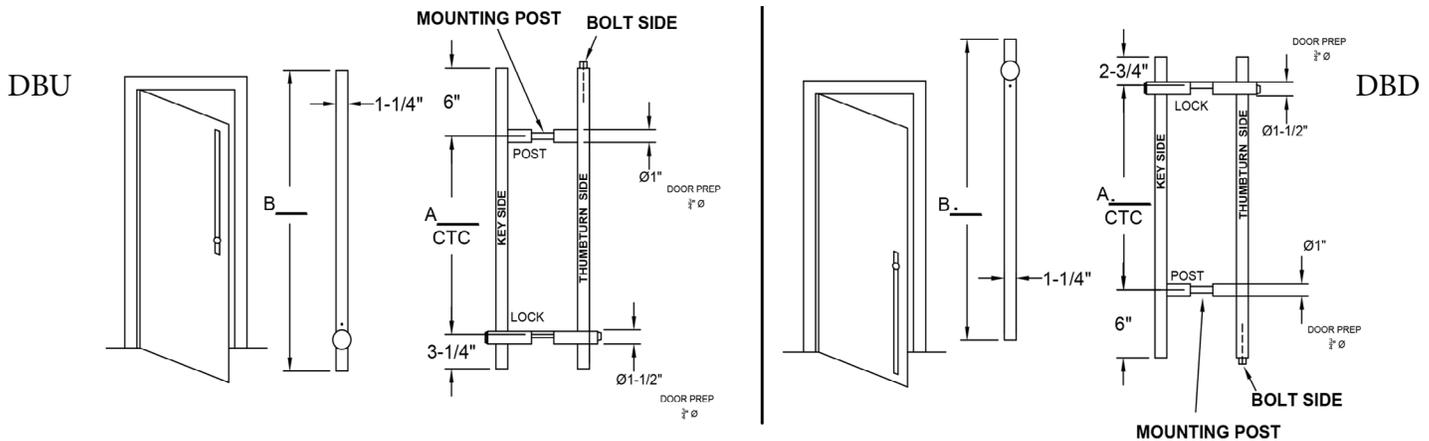
**NOTE: CYLINDER MUST BE LOCATED 34"-48" ABOVE FINISHED FLOOR TO MEET ADA REQUIREMENTS. CALIFORNIA ADA REQUIRES CYLINDER TO BE LOCATED 36"-46" ABOVE FINISHED FLOOR.**
