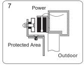
After the magnet attracts the armature plate, adjust the Z bracket to fit the door.
