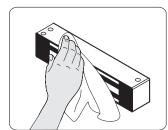
Wipe the surface of magnet lock with anti-rust oil regularly.
