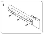
Find a mounting position on the door frame for the L bracket. Make sure that the door can still be closed.
