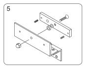
Attach the armature plate and washers to the Z bracket assembly.
