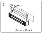
Use the fixing bolts to tighten the magnet on L bracket.
