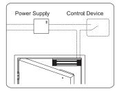
The electromagnet locks are fail-safe, therefore it may be required that the UPS remain locked during power failure.
