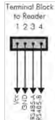
Because of the line resistance, certain cable lengths should not be exceeded. The data wires 485-A and 485-B should be twisted together, particularly when using long cables (twisted pair cable).
