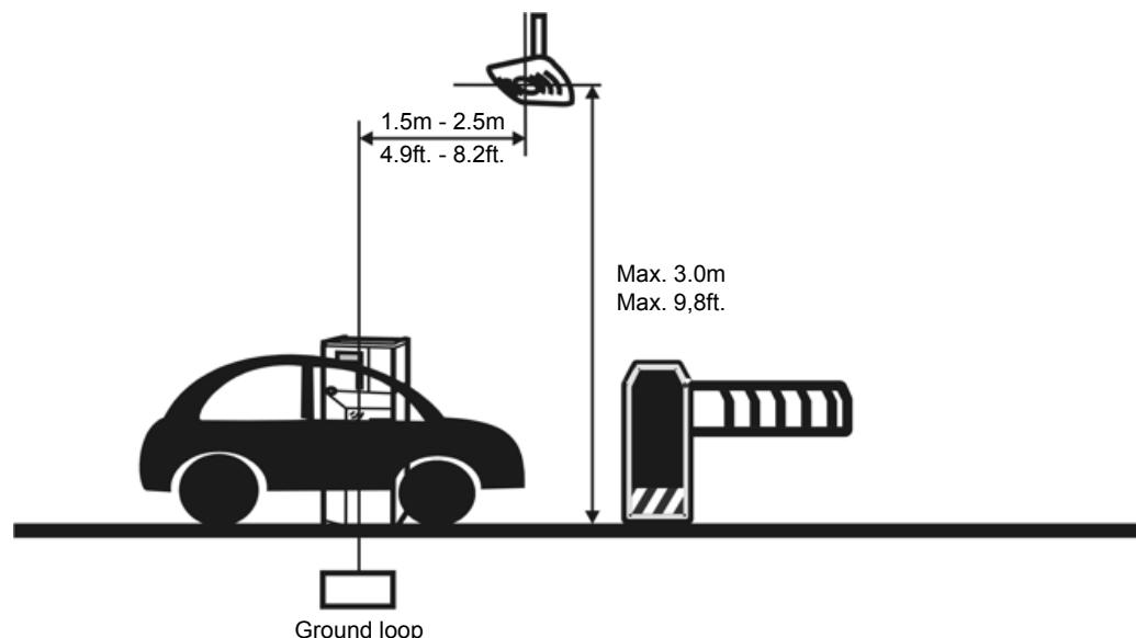
**Note: The antenna beam of the reader shall in no case be restricted by objects above or below the reader. Flush mounting is not recommended! If other types of vehicles (trucks, small cars etc) need to be identified, the reader must be installed and aligned individually.**
