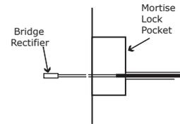
**STEP 5:** Connect the Bridge Rectifier to the plug exiting the mortise chassis.
