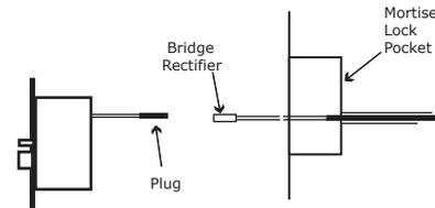
**STEP 6:** Carefully slip the connected mortise lock chassis into the mortise pocket paying close attention not to pinch any wires.
