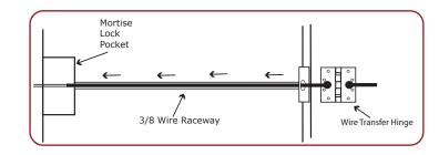
**4.** Connect the wires exiting the mortise pocket to the Bridge Rectifier (included).
