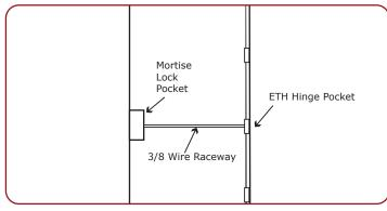
Screw the ETH hinge to the door. At this time <u>DO NOT</u> connect the hinge wires on the jamb side to the wires coming from the power supply.
