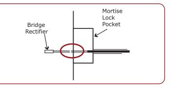
Carefully slip the connected mortise lock chassis into the mortise pocket paying close attention not to pinch any wires.
