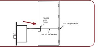
**B** Connect the wires from the power supply at the ETH hinge on the jamb side. Connect the hinge to the jamb.
